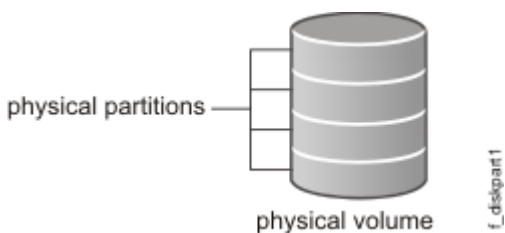
Figure 5: Physical partitions on a physical volume
